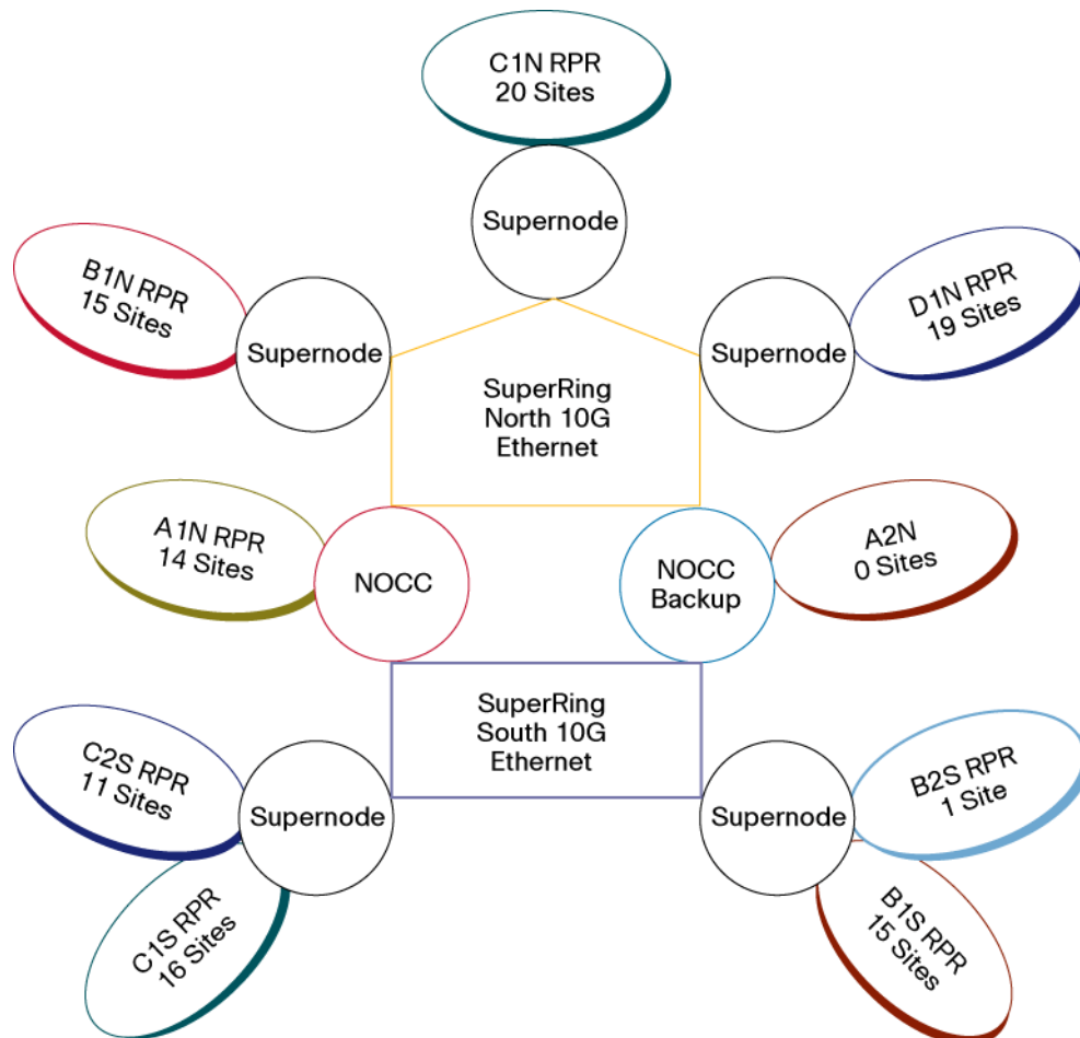
Figure 1. AISD GAATN Network Ring Topology
